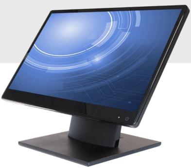
This simple reliable system is based on an ARM (Advanced RISC\* Machine) processor and thus perfectly meets the needs of the POS market in terms of Android requirements, guaranteeing an easy access to Google Play Store thanks to its GMS certification (Google Mobile Services).
